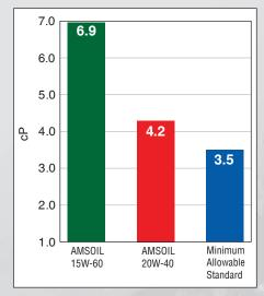
The High-Temperature/High-Shear Viscosity Test (ASTM D5481) measures a lubricant's viscosity under severe high-temperature and shear conditions, similar to severe operating conditions experienced by motorcycles. Higher values indicate improved wear protection.
