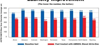
The ASTM D975 diesel fuel standard specifies a wear scar below 520 µm in ASTM D6079 testing, while the Engine Manufacturers Association (EMA) specifies a wear scar below 460 µm. Testing reveals AMSOIL Diesel All-In-One provides significant lubricity improvement in diesel fuels found across the U.S., delivering improved wear protection.
