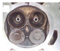
Combustion chamber before P.i. treatment.
