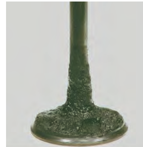
Picture D - Intake valve before P.i. treatment
