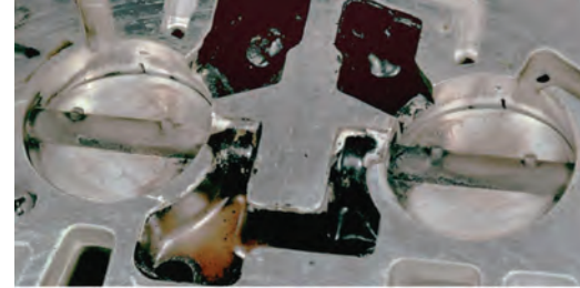
Picture K - Carburetor plates after P.i. treatment
