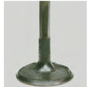
Picture E - Intake valve after P.i. treatment
