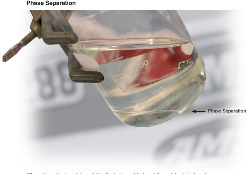
When ethanol/water mixtures fall to the bottom of fuel containers, it leads to lean-burn situations. Quickshot helps keep water molecules dispersed to prevent phase separation.
